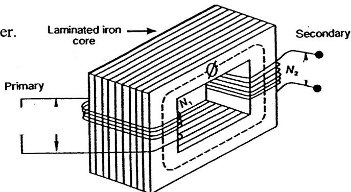
1. Would the diagram of the transformer represent a step-up or a step-down transformer? Explain your answer. (2 marks)
